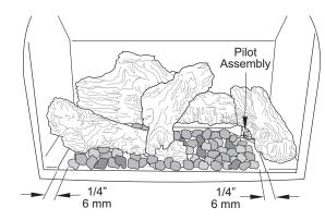
Figure 24. Position embers loosely and maintain 1/4" clearance from the burner skirt edges.
